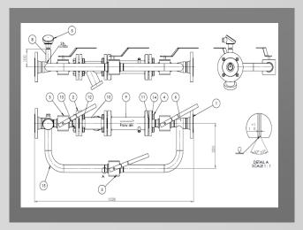
MGO combustion is upgraded to flow feedback by installing marine proved KRAL flowmeter, ensuring exact and precise feedback in fractions of liter. Such precise feedback ensures more precise information for ACC (Automatic Combustion Controller), which results in superior combustion during MGO operation.
